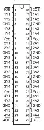
The 74ACT16240 is packaged in TI's shrink small-outline package, which provides twice the I/O pin count and functionality of standard small-outline packages in the same printed-circuit-board area.
